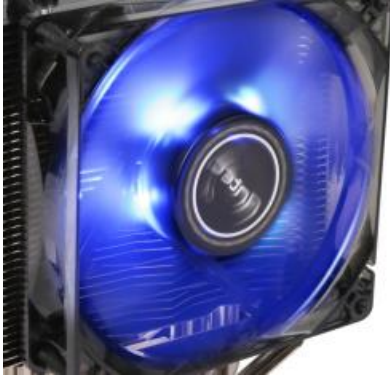
9cm blue LED+4Pin temperature controlled fan
